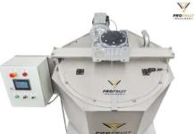
Multi-purpose jam cooker is double-walled and entirely made from stainless steel. Machine has an integrated mixer with specially made scrappers which prevent product from sticking. The jam cooker has adjustable speed as well as fully automatic temperature and cooking time control. The machine also has an integrated touchscreen panel with ability to set the recipes, time, temperature and mixing speed. Therefore, it significantly easies the cooking process and reduces the workload.
